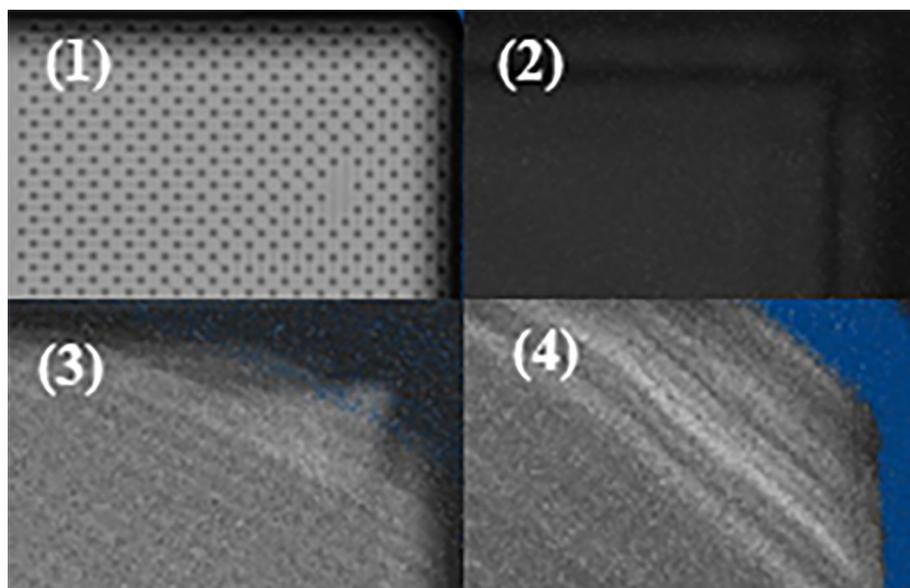
Fig. 14. FlipChip analysis in water (1), FC-43 (2), D02 (3) and HT80 (4) at 20 °C, using a 110 MHz transducer.
