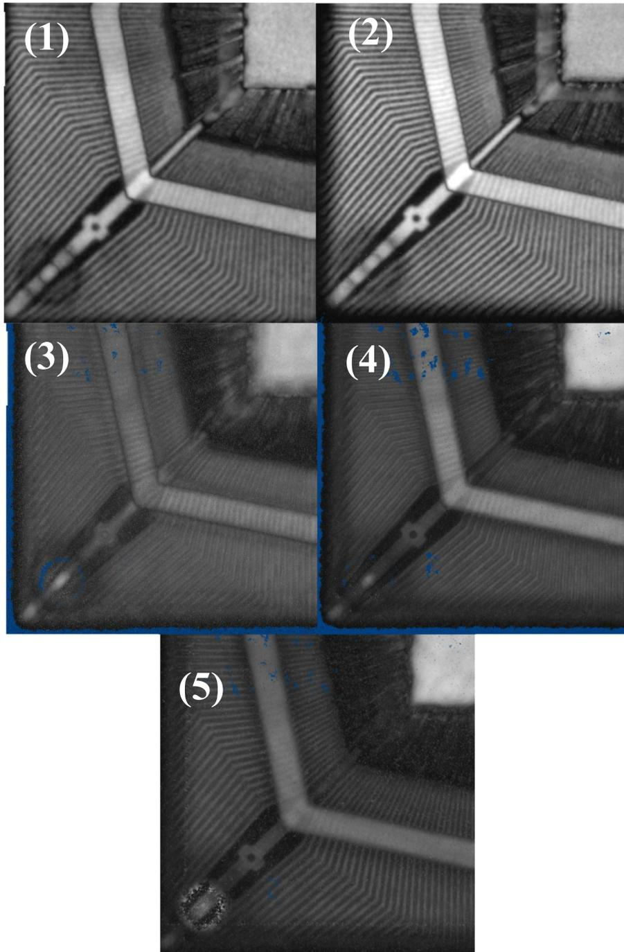
Fig. 11. PQFN analysis in water (1), isopropanol (2), FC-43 (3), D02 (4) and HT80 (5) at 20 °C, using a 35 MHz transducer.
