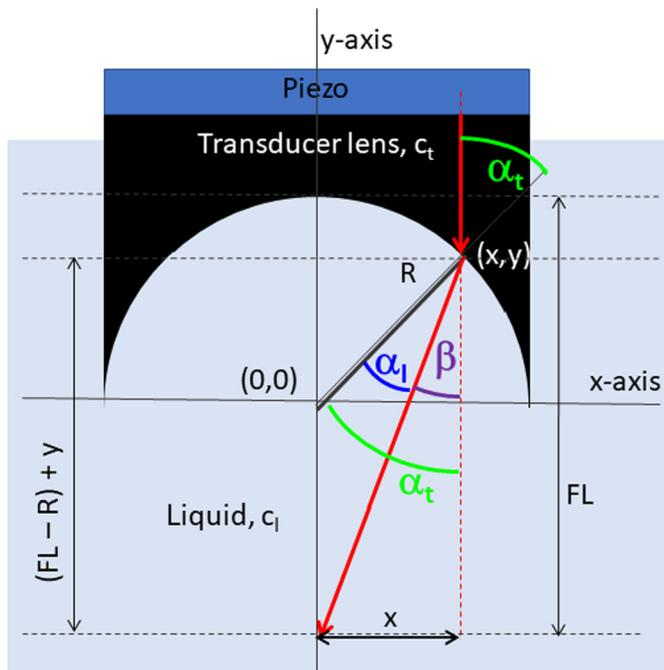
Fig. 6. Schematic representation of a plane sound wave, travelling through the transducer lens and being focused by the curved lens-liquid interface.  $c_t$ ,  $c_l$ : sound velocities in the transducer lens and the coupling liquid, respectively.
