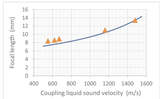
Fig. 7. Calculated variation of the focal length of the used 15 MHz transducer ( $FL$  13.4 mm in water) with the coupling liquid's sound velocity (line). An estimated sound velocity of 2600 m/s is used for the transducer's epoxy lens. Markers: experimentally determined focal lengths with the five coupling liquids used in this study.
