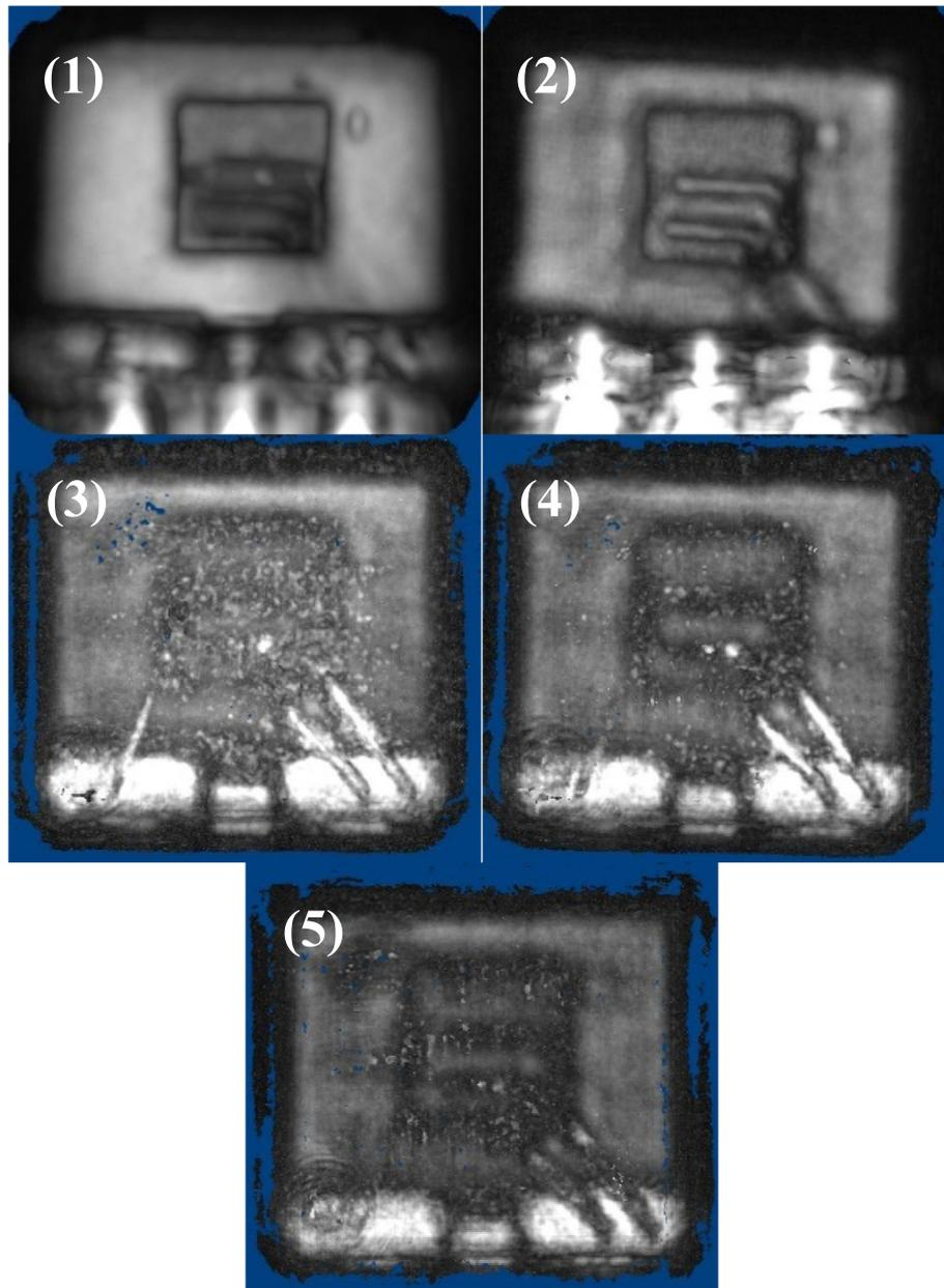
Fig. 10. Top side analysis of the TO component by a 15 MHz transducer, in water (1), isopropanol (2), FC-43 (3), D02 (4) and HT80 (5) at 20 °C.
