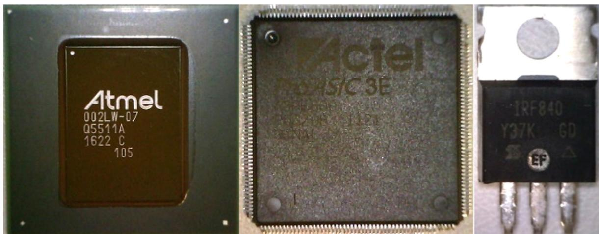
**Fig. 9.** The samples used in this study are reference samples for long-term reliability analysis at French national space research center CNES. From left to right: FlipChip, PQFN208, TO.
