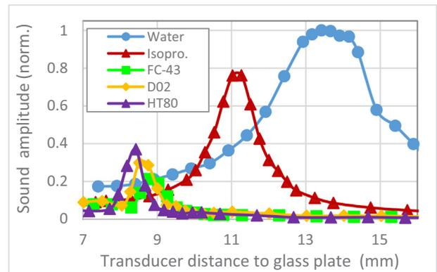
Fig. 8. Reflected ultrasound amplitude vs. transducer-to-glass plate distance for the five coupling liquids of this study. For each liquid, the measured sound amplitude is divided by the reflection coefficient of the sound on the respective liquid/glass interface.
