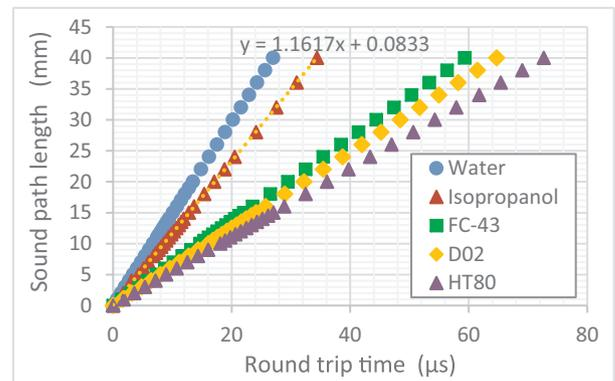
Fig. 3. Measurement of the sound path length vs. pulse round trip time in deionized water, isopropanol, FC-43, D02 and HT80, at 20 °C liquid temperature. The evaluation of the sound velocity by linear regression is shown for isopropanol.
