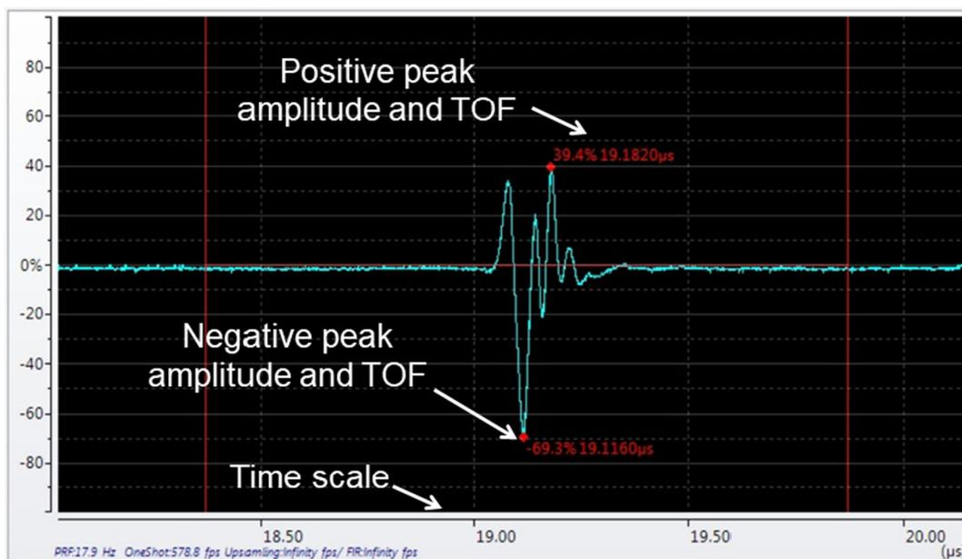
Fig. 2. Example of a received sound pulse. The round-trip time (time of flight – TOF) of the pulse from the transducer to the sample and back is displayed on the abscissa. The ordinate shows the peak amplitude as percentage of the full scale.
