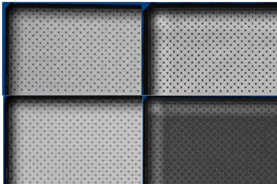
Fig. 13. FlipChip analysis in water (left) and isopropanol (right) at 20 °C (top) and 40 °C (bottom) with a 110 MHz transducer.
