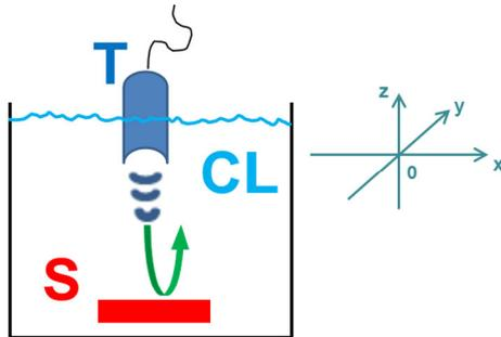
Fig. 1. Experimental setup. T: transducer. CL: temperature stabilized coupling liquid. S: sample.
