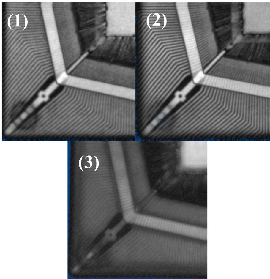
Fig. 12. PQFN208 analysis in water (1), isopropanol (2) and FC-43 (3) at 40 °C, using a 35 MHz transducer.
