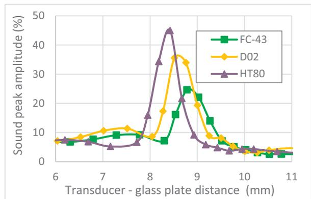
Fig. 5. Reflected ultrasound amplitude vs. transducer-to-glass plate distance with FC-43, D02 and HT80 as coupling liquids. The nominal focal length of the transducer in water is 12.7 mm.
