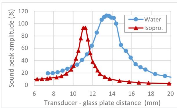
Fig. 4. Reflected ultrasound amplitude vs. transducer-to-glass plate distance with water and isopropanol as coupling liquids. The nominal focal length of the transducer in water is 12.7 mm.
